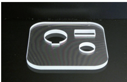
Laser cut glass in different sizes and shapes (glass thickness 4 mm)
