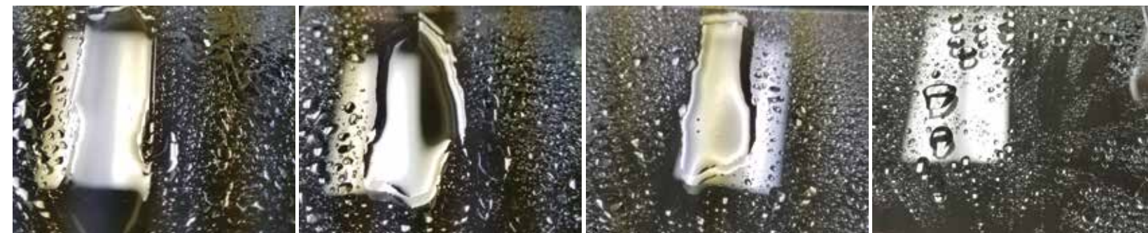
EnduroShield® Glass Coating Visible wear after 1,000 abrasion cycles Fail
