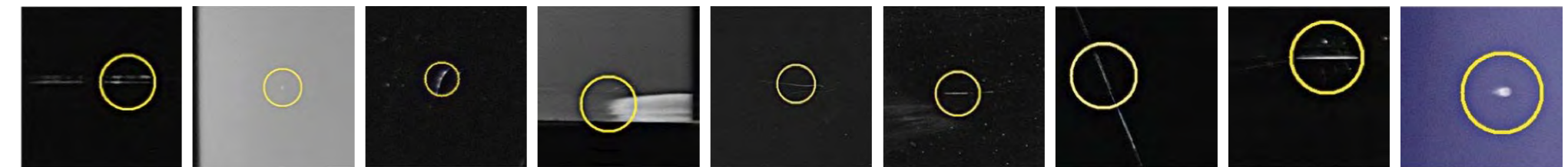
▲ Detects pinholes, arc marks, edge grind skips and misses, skip scratches and cluster defects
