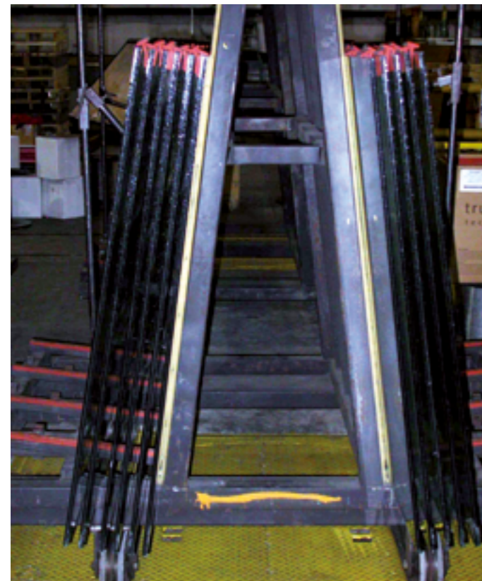
FIG 24 • Properly racked laminates
