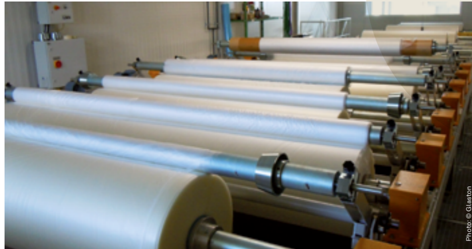
Storage room for PVB interlayer
