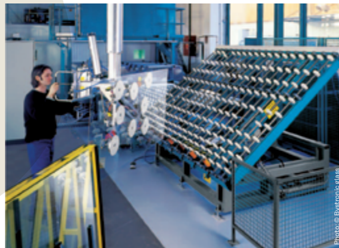
• Unloading of glass from rack before washing
