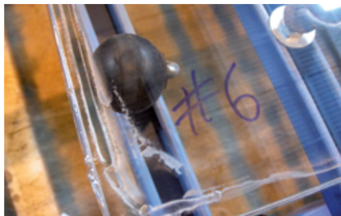
FIG 18 • Trapped air in trailing edge
