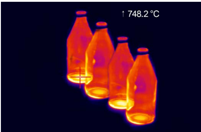
Hot spot detection in glass bottle production
