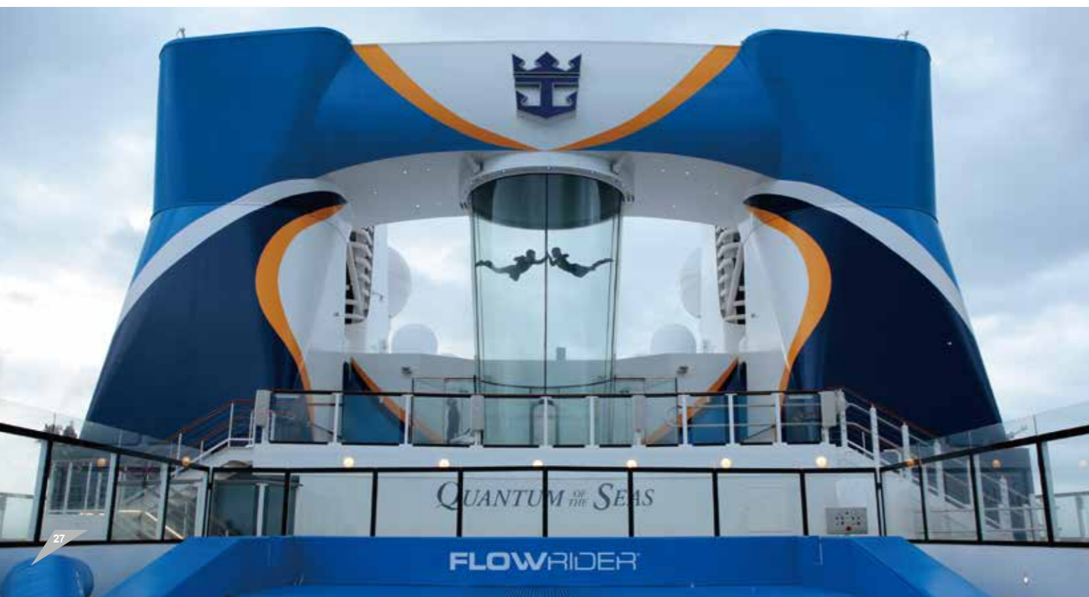
▼ Wind Tunnel Cabin of "Quantum of the Seas" Cruise Glass makeup: 10mm super clear glass curved tempered HST (outer layer)+1.52SGP+10mm super clear glass curved tempered HST+2.28 SGP+10mm super clear glass curved tempered HST Furnace used: AC15E128
